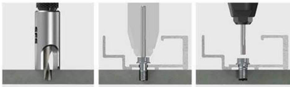
Figure 7 –patte-agrafe coulissante et fixe
